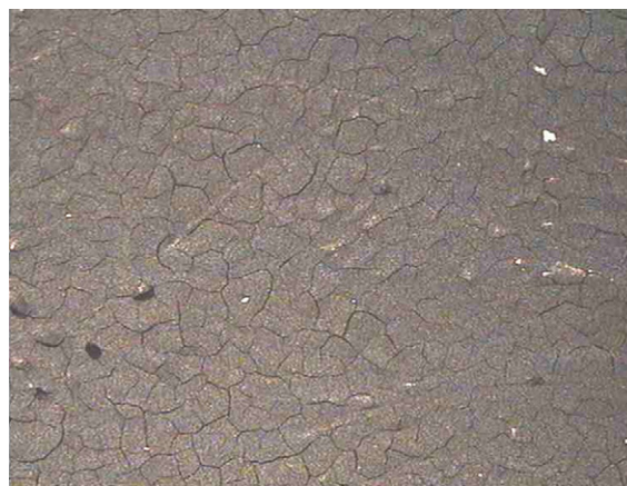
Fig. 6. Stereo optical micrograph (150 \times ) of HMS/Pt/LPG dispersed upon Ti fibre mesh electrode substrate.
